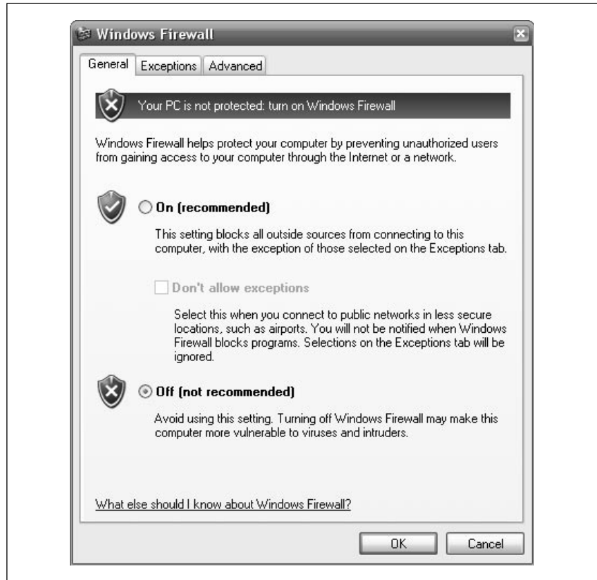
Figure 5-11. The Windows Firewall, which is turned on by default in Windows XP Service Pack 2, is known to cause problems.
