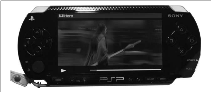
Figure 3-5. The Display control panel places the name of the movie in a bar across the top and a progress bar along the bottom
