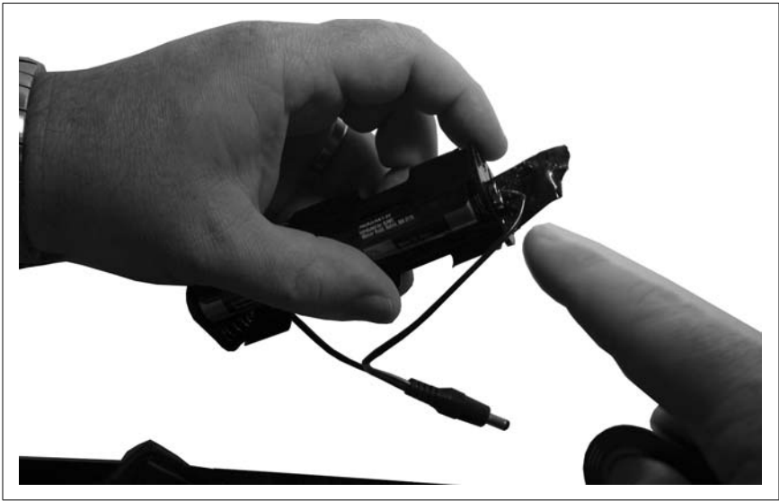
Figure 2-39. Taping the negative line to the negative plug on the battery holder
