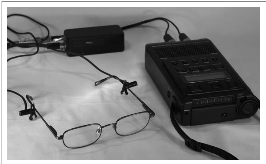
Figure 3-10. A set of binaural microphones on glasses, attached to a Marantz 660
