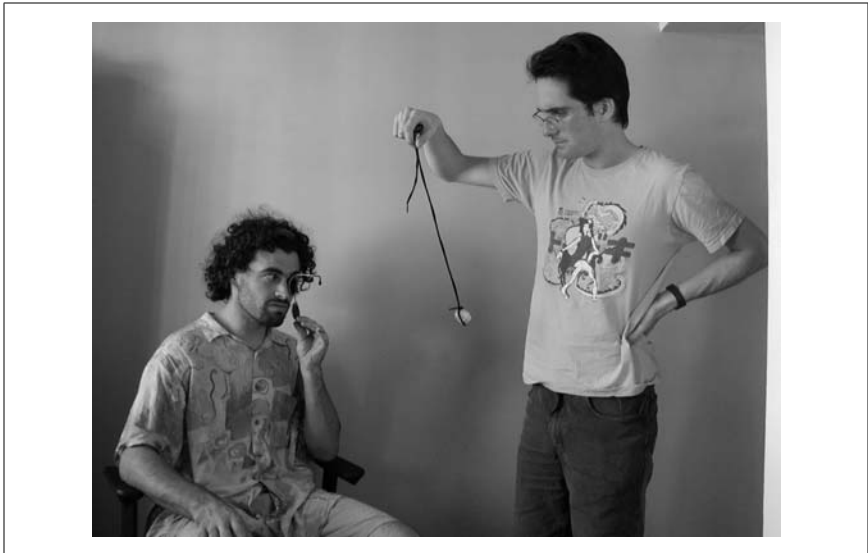
Figure 2-21. Matt and Tom use sunglasses and a pendulum made out of a bootlace to test the Pulfrich Effect
