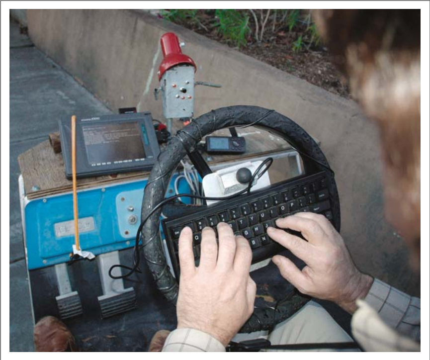
Figure 5-33. A homebrewed geo-annotation device with custom “little man” keyboard
