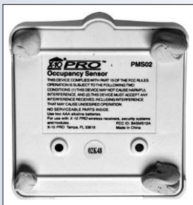
Figure 3-3. Poster adhesive is an easy way to secure your motion detectors.
