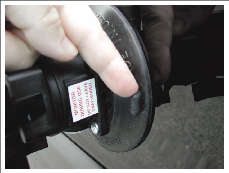
Figure 3-6. Pull on the tab firmly to release the vacuum
